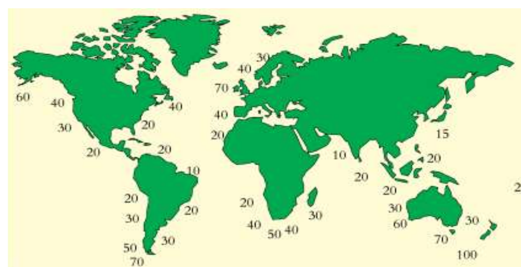
World-wide estimate of wave energy in kW/m of coastline. By T. Thorpe 2005
