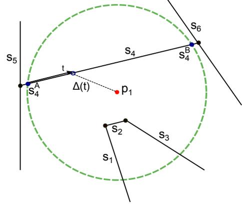
Fig. 3.  $S_4^A$  and  $S_4^B$  are the end points of the portion of  $S_4$  that falls inside the error region, which we name as  $\bar{S}_4$ . This line segment is parameterized with parameter  $t$ , and the distance from a point on  $\bar{S}_4$  to  $p_1$  is formulated by  $\Delta(t)$ .
