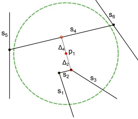
Fig. 2. Circular error region defined around GPS point,  $p_1$ . Segments  $S_1, S_2, S_3, S_4$  are the candidate road segments for  $p_1$ .  $\Delta_2$ , and  $\Delta_4$  are the shortest distances from  $p_1$  to segments  $S_2$ , and  $S_4$ , respectively.  $\Delta_2 \approx \Delta_4$ .
